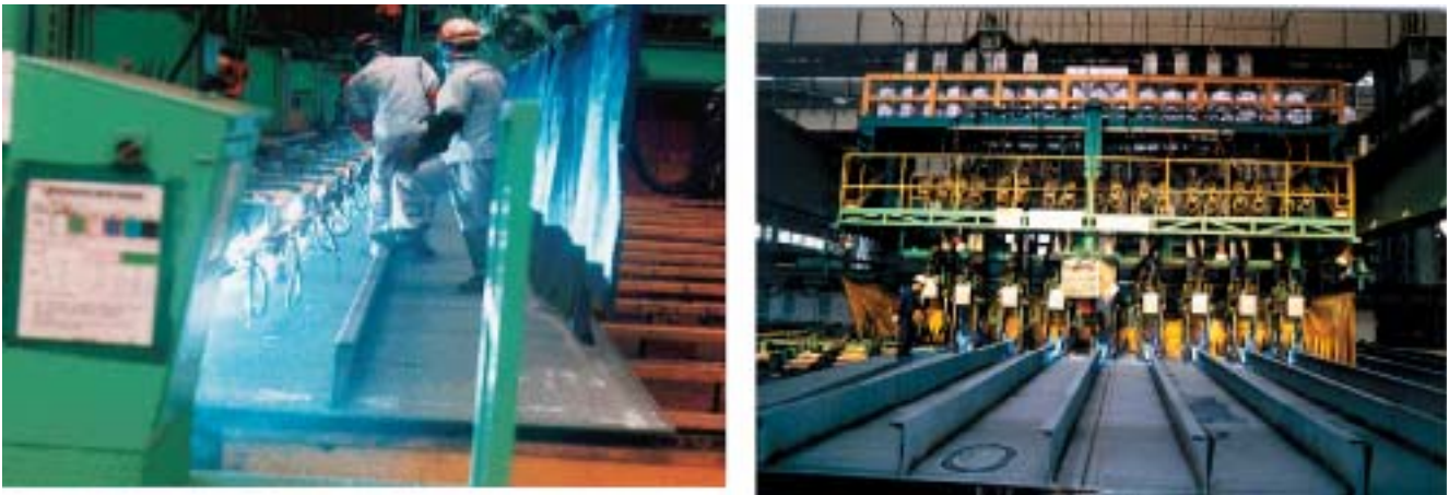
Figure 1. Mechanised system at shipyard (left: gantry type – single torch, right: TAMA type – twin tandem with 24 torches).
