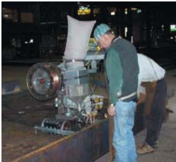
Figure 1. Capitol Steel uses the A6 Tandem Mastertrac to make horizontal fillet welds up to 7/16" (11 mm).
