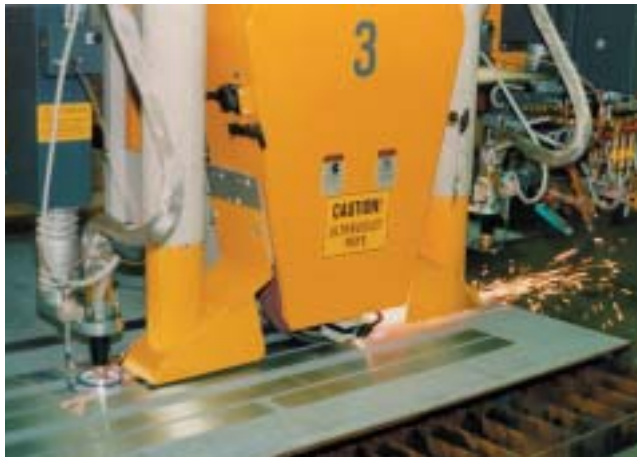
Figure 5. Grinding device for surface cleaning.
