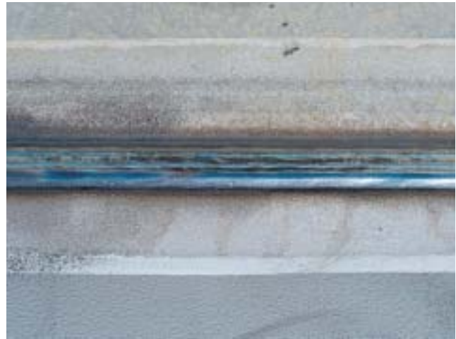
Figure 4. Capping passes of horizontal joint welded by 2 Circotech with OK 12.32 and OK Flux 10.71. The excellent weld appearance and blending of the three passes is readily apparent.
