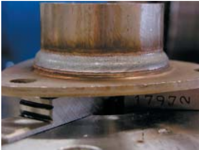
Figure 1. The results using the metal-cored wire, PZ 6470 1.2 mm. Note the smooth transitions between the welds and the parent material, the clean weld surface and the absence of spatter.
