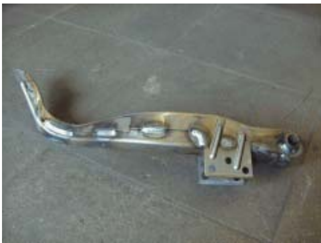
Figure 2. A typical thin-plate application from a supplier to the automotive industry. Welded with the new metal-cored wire.
